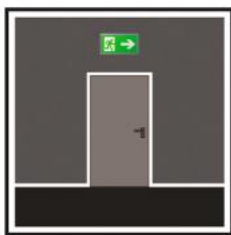
at each emergency exit door
