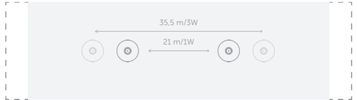
simulation for two luminaires and min 1 lx (distance)
