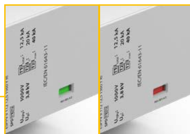
Optical indicator (red window colour - should be replaced; green window colour - functional).
