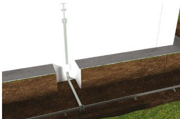
An example of grounding using a Tape Conductor.
