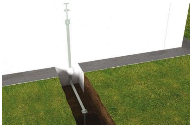
An example of grounding using an Earthing Electrode
